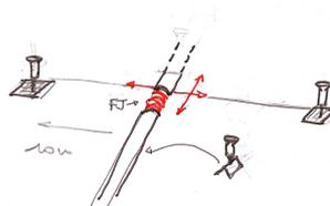
These markers shall be deployed 10m each side of an easily identifiable point of the pipe/ structure, in order to be able to detect small displacement using either top or lateral visual alignment or acoustic metrology using in this case, a saddle placed on the pipe.
